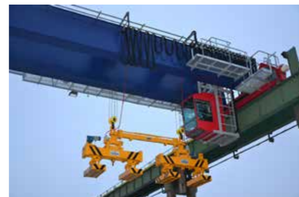
7 cranes with magnetic beams used for handling metal sheets and metal profiles (Customer „BLRT group“)
