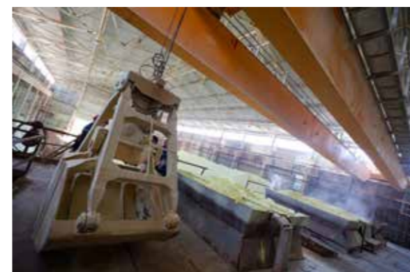
Bridge crane with grab SWL 5t used for handling sulphur (Customer „GrodnoAzot“)
